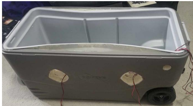
Fig. 3.6: Running Wires Through Interior Panel
