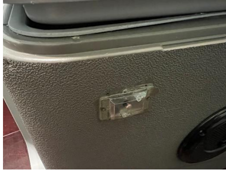
Fig. 3.11: Photosensor Mounted on Exterior of Cooler
