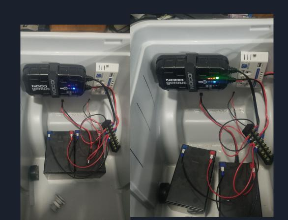
Charging confirmed both sides, 120V AC & 12V DC Battery Charging
